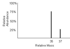
75% of the sample consist of chlorine-35, and 25% of the sample is chlorine-37.
